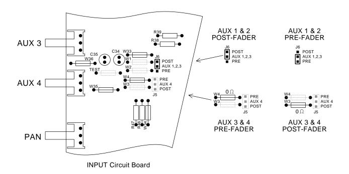
Aux 1 & 2: These sends are factory set for post-fader operation. To change Aux 1 & 2 to pre-fader (on a given channel), move jumper strap J6 to the 'PRE' position (see diagram). Aux 1 & 2 are changed as a pair (not individually). Channels must be modified individually.
