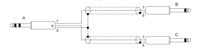
Two other uses for this Patch cable are: 1) To provide a stereo line input to the Return 1 & 2 jacks from stereo effects devices with separate left & right outputs (Tip B connects to the left output of the effects device and Tip C connects to the right output of the effects device). 2) To provide a stereo line output from the Headphones jack for connecting to a stereo sound system (Tip B is the left output and Tip C is the right output).
